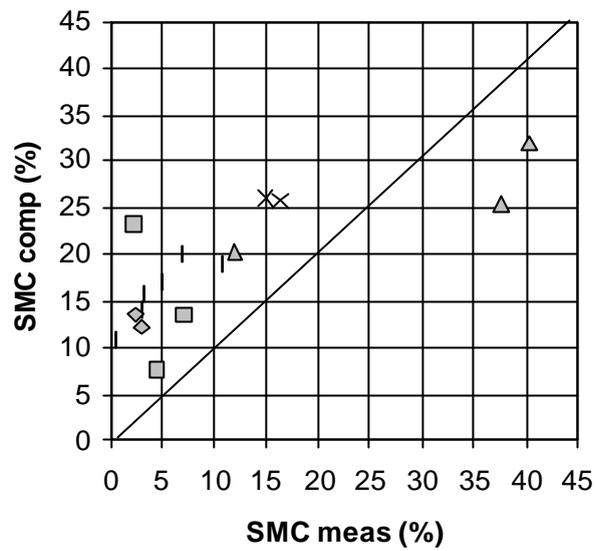
Fig. 2 - SMC % estimated with the algorithm as a function of SMC % of the first 5 cm layer measured on ground. The line represents the 1:1 line. Symbols refer to different crop types:  $\square$  = alfalfa,  $\blacktriangle$  = bare soil,  $x$  = sunflower,  $\blacklozenge$  = wheat.
