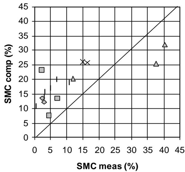
Fig. 2 - SMC % estimated with the algorithm as a function of SMC % of the first 5 cm layer measured on ground. The line represents the 1:1 line. Symbols refer to different crop types:  $\square$  = alfalfa,  $\blacktriangle$  = bare soil,  $\times$  = sunflower,  $\blacklozenge$  = wheat.
